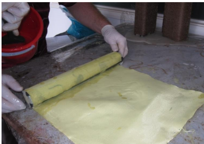
Figure 6: Typical Picture, Hand Lay-Up Fabrication Method
