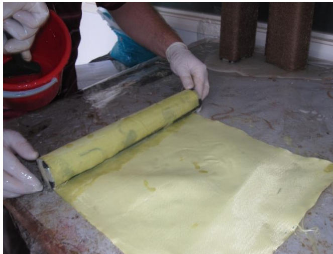
Figure (2) : Typical picture, hand lay-up fabrication method
